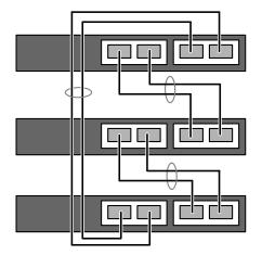
1-port interface modules do not support port aggregation in the IRF. When 1-port interface modules are connected for an IRF, the port of MOD 1 can only be connected to the port on MOD 2, as shown by callout 1 in <u>Figure 3-30</u>; when a 1-port interface module is connected to a 2-port interface module for an IRF, the port of MOD 1 can only be connected to the right port of the 2-port interface module, as shown by callout 2 in <u>Figure 3-30</u>.
