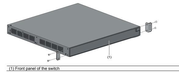
**Step4** Place the switch horizontally in a proper position, and fix the other end of mounting brackets to the front brackets with screws and captive nuts, as shown in Figure 3-5.
