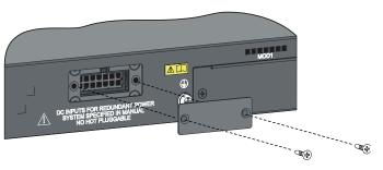
Figure 3-20 Connect an RPS power cord (1)
