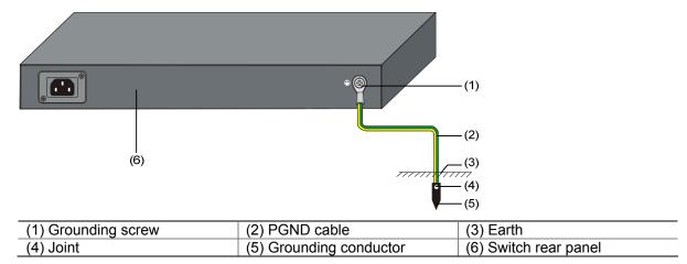
Figure 3-13 Ground the switch by burying the grounding conductor into the earth
