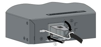
Figure 3-18 Connect an AC power cord to a vertical AC power socket (1)
