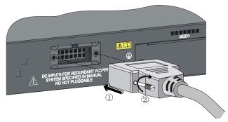
Figure 3-21 Connect an RPS power cord (2)
