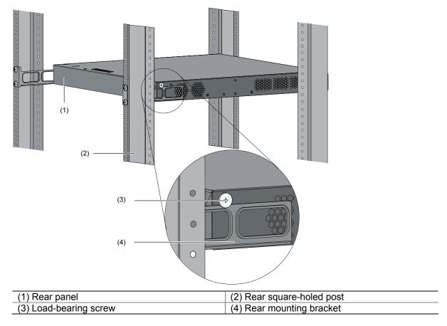
Step7 Fix the other end of the front mounting brackets to the front brackets with screws and captive nuts and ensure that front and rear mounting brackets have fixed the switch in the cabinet securely, as shown in <u>Figure 3-10</u>.
