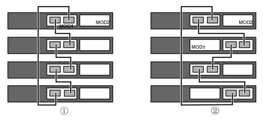
• When 2-port interface modules are adopted in an IRF with ports operating in the aggregation mode, ports of MOD 1 can only be connected to ports of MOD 2, and the locations of the ports of the interface modules are not limited.
