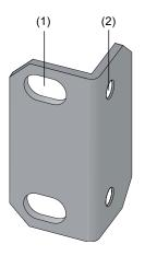
(1) Screw hole used to fix the mounting bracket to the cabinet (Use one M6 screw)(2) Screw hole used to fix the switch to the mounting bracket
