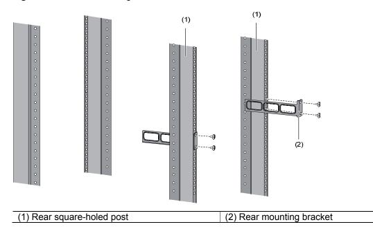
Figure 3-7 Fix rear mounting brackets
