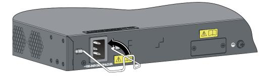
Figure 3-19 Connect an AC power cord to a vertical AC power socket (2)
