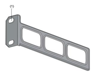
(1) Screw hole used to fix the mounting bracket to the cabinet (Use one M6 screw)
