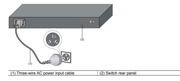
Figure 3-14 Ground through an AC power PE wire
