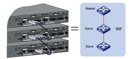
Figure 3-27 The ring connection mode
